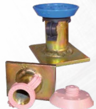
Details: Socket, high grade precision steel tube, welded onto flat steel ST 37-1, black or galvanized; data clip, synthetic material; recess plate, synthetic material
