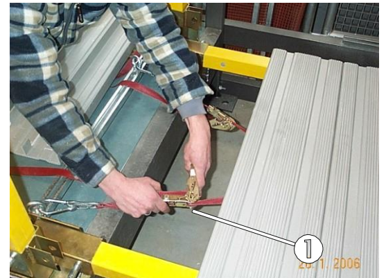
Fig. 33: Equal application of maximum tension force
