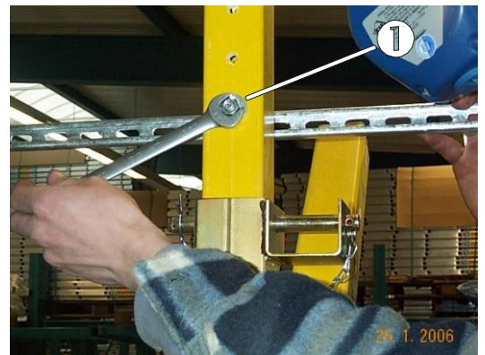
Fig. 41: Inserting the washer to distribute the force
