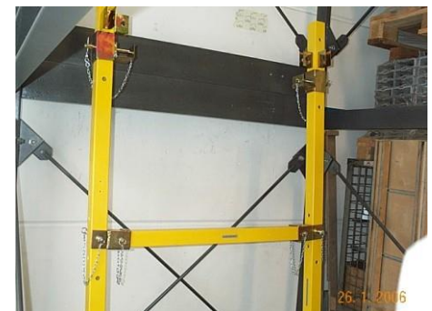
Fig. 52: Locking pins for securing the long bar
