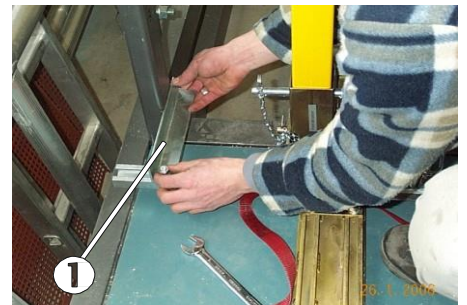
Fig. 43: Attaching the second L angle
