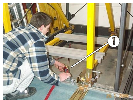
Fig. 30: Pre-tension the belts
