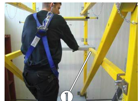
Fig. 77: Laying the upper floor panels
