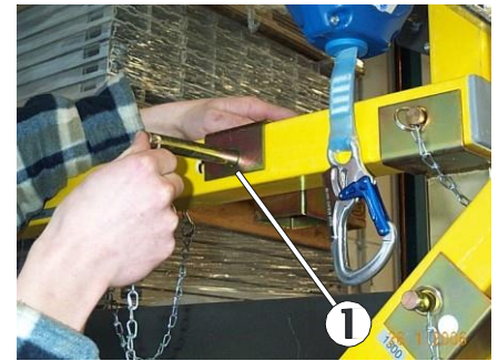
Fig. 75: Determining the correct insertion position
