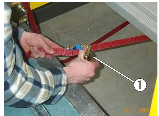
Fig. 27: The ratchet on the clamping belt is used to generate light preliminary tension
