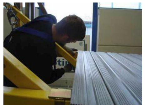
Fig. 82: Tube clamps to prevent the floor panels from slipping
