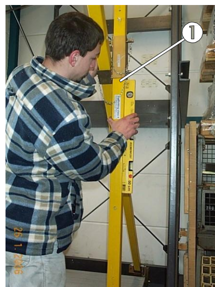
Fig. 37: Attaching the short piece of the tension belts
