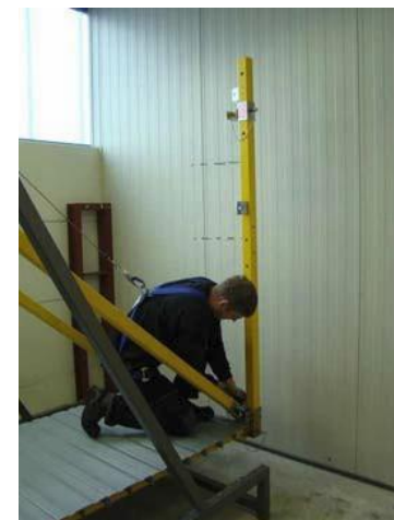
Fig. 46: Pin locking device for the rear vertical rail stanchion
