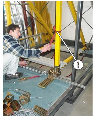
Fig. 25: Loosening the second half of the tension belt
