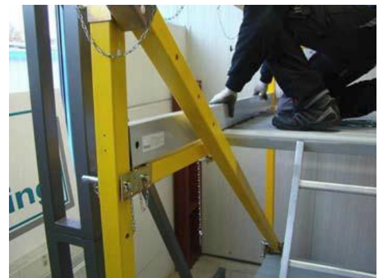
Fig. 90: The locking pin is inserted from above
