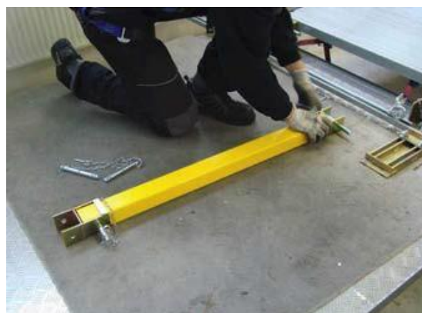
Fig. 49: Pre-assembly of the front bar
