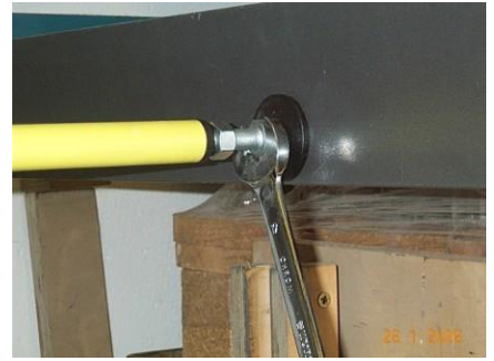
Fig. 71: Adjustable foot for vernier adjustment of length
