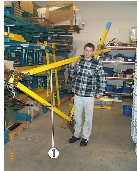
Fig. 12: Transporting the triangular structural part
