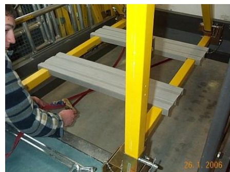
Fig. 29: Required gap of panel from ratchet
