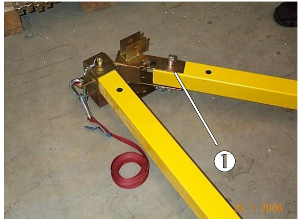
Fig. 9: Attaching the diagonal profile
