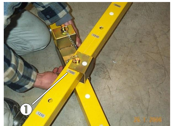
Fig. 9: Attaching the diagonal profile
