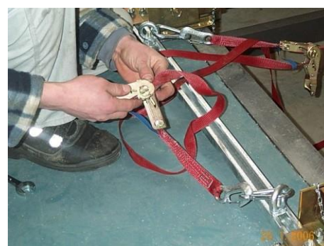
Fig. 29: Required gap of panel from ratchet
