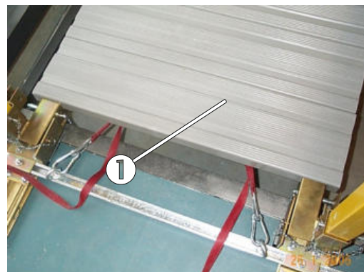
Fig. 37: Attaching the short piece of the tension belts
