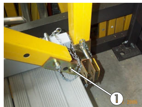
Fig. 67: Mounting the toeboard at the rear with a long locking pin
