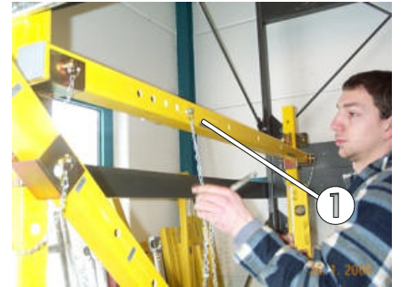
Fig. 60: Attachment of inner and outer tube with a short locking pin
