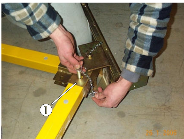
Fig. 6: Vertical and horizontal sides of triangles, connected to the left-hand threshold bracket
