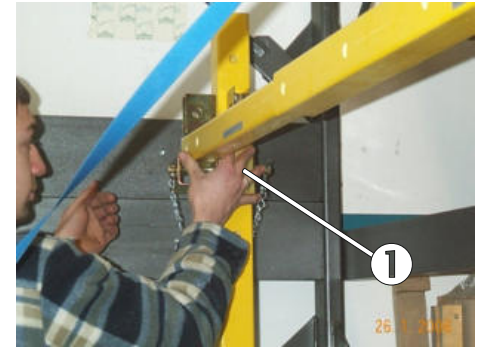
Fig. 55: Rear bar must be held into place during mounting process
