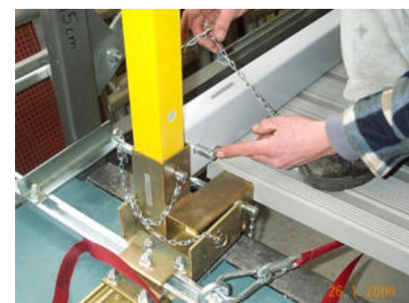
Fig. 67: Mounting the toeboard at the rear with a long locking pin
