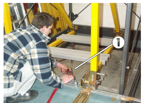
Fig. 30: Pre-tension the belts
