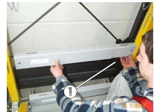
Fig. 70: Mounting the front midrail
