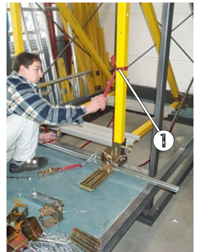
Fig. 25: Loosening the second half of the tension belt
