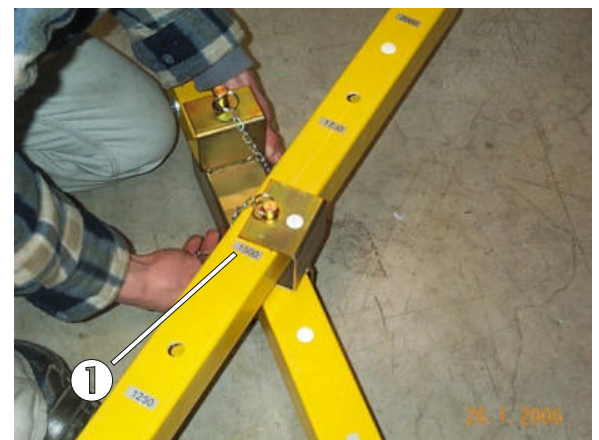
Fig. 10: Setting the platform depth
