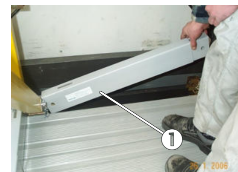
Fig. 69: Mounting the front toeboard
