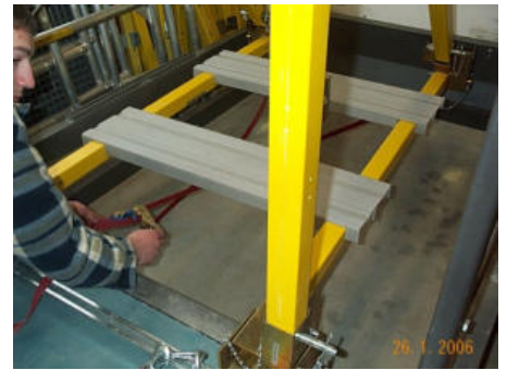
Fig. 29: Required gap of panel from ratchet
