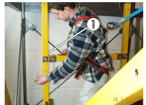
Fig. 52: Locking pins for securing the handrail
