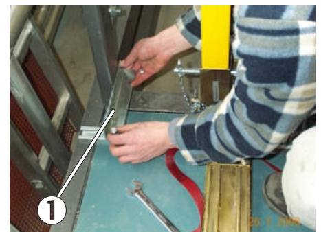
Fig. 43: Attaching the second L angle
