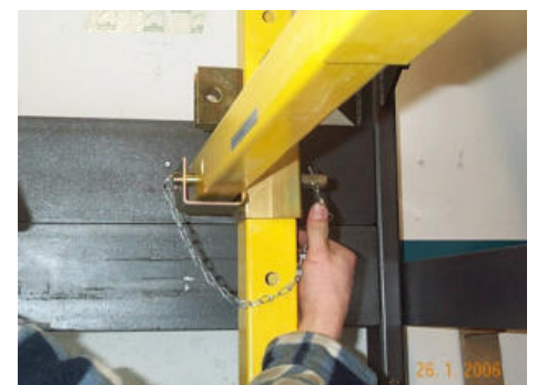
Fig. 56: Front fastening bolt for securing the bar
