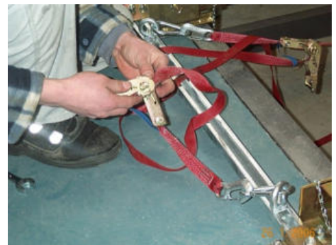
Fig. 29: Required gap of panel from ratchet
