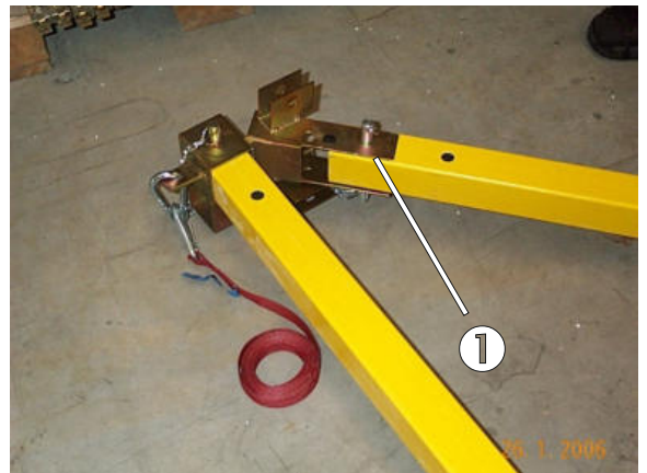
Fig. 9: Attaching the diagonal profile
