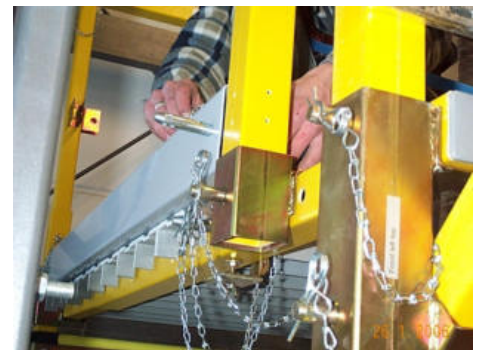
Fig. 97: The locking pin is inserted from above
