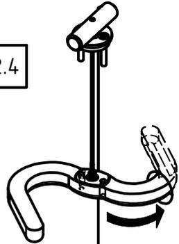
EN: Both screws have to be tighten parallel
