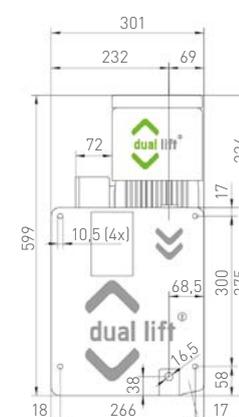
**TREUILS POUR PERSONNES SELON EN1808 AVEC BOÎTIER DE COMMANDE SUSPENDU ENFICHABLE SUR LE TREUIL CÂBLE 2,5M**
