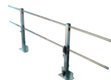
**FOLDABLE VERSION:** fully galvanised, with fixing material; **Height Variant 1:** 0.70m, with 2 vertical supports and 2 horizontal bars; **Height Variant 2:** 1.10m, with 2 vertical supports and 2 horizontal bars; **Length:** 0.93–1.62 m (hand and knee rails can be cut down to the required size on site). A twin contact protection ensures the surveillance of both positions.
